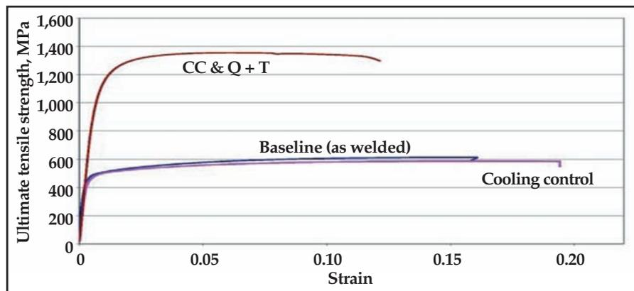
**Fig. 15 — Typical stress-strain plots for seam-welded 28.6 mm diameter × 0.5 mm Type 410 SS tubing.**
