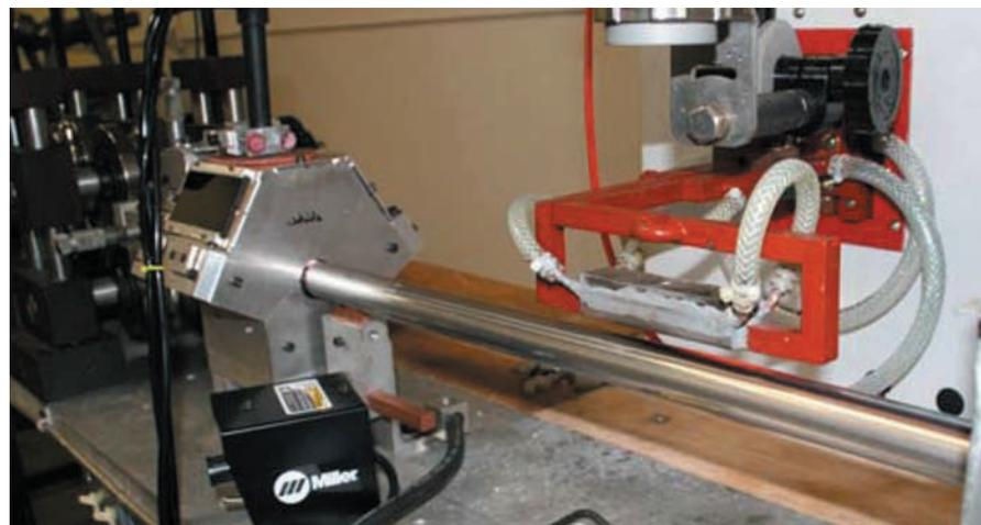
**Fig. 13 — Tube mill weld-zone with inductor installed; material travel from left-to-right.**
