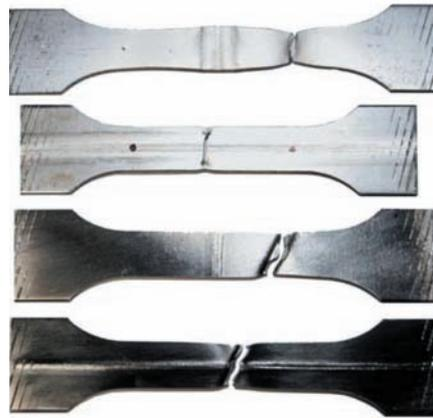
Fig. 10 — Typical tensile-test weld specimen fracture locations. From top: transverse (T), annealed base metal; longitudinal (L), annealed base metal; T, post-weld CC and Q+T; L, post-weld CC and Q+T.
