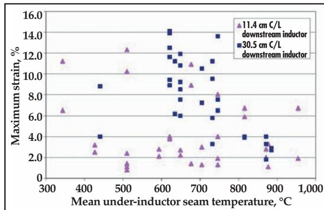
Fig. 7 — Maximum elongation versus mean under-inductor weld seam temperature for varying downstream inductor coil distances; longitudinal weld seam specimens include all gauges.
