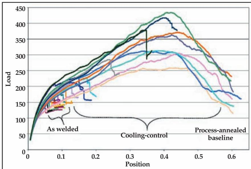
Fig. 6 — Comparison of 3-point longitudinal face-bend test load-position data for various process conditions. Modified ASTM E190 guided bend test for ductility of welds. Bend Radius = 4t; t = 1 mm.
