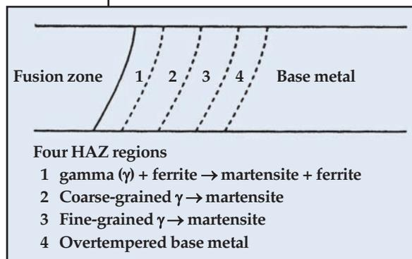
**Fig. 1 — Four HAZ regions in a martensitic stainless steel weld<sup>[1]</sup>.**
