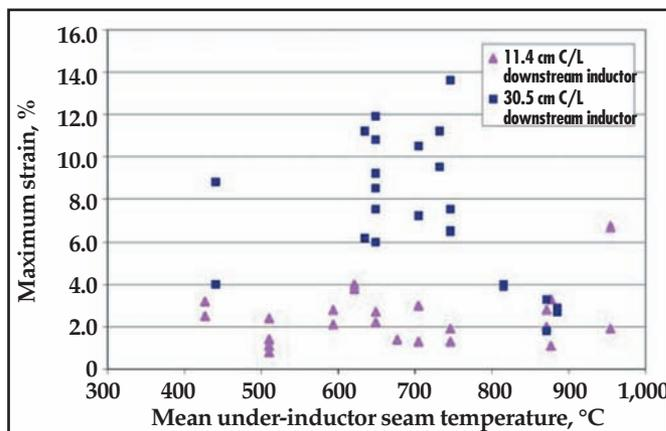
Fig. 8 — Maximum elongation vs. mean under-inductor weld seam temperature for varying downstream inductor coil distances; longitudinal weld seam specimens 1 and 2 mm only.
