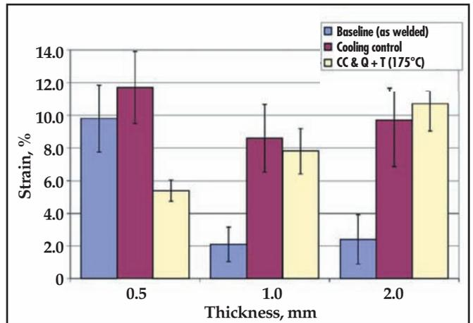
Fig. 11 — Comparison of maximum strain at fracture for optimum process conditions; DIN EN 895 longitudinal tensile specimen, average results for 62 trials.
