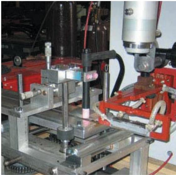
Fig. 2 — Seam weld/cooling-control test apparatus.
