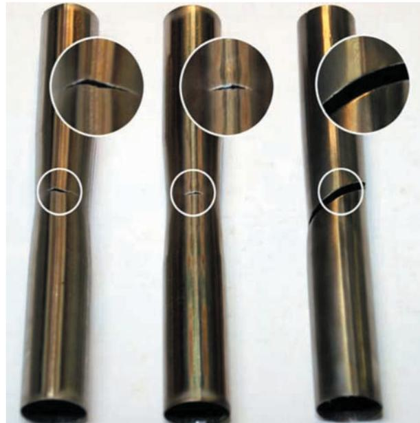
Fig. 17 — Typical tensile test tube specimens; from left: as welded; cooling-controlled; C.C. Q+T hardened.
