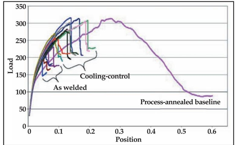
Fig. 5 — Comparison of 3-point longitudinal face-bend test load-position data for various process conditions. Modified ASTM E190 guided bend test for ductility of welds. Bend Radius =  $2t$ ;  $t = 1$  mm.
