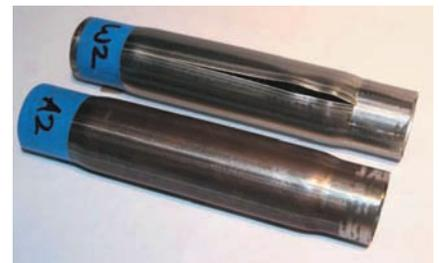
Fig. 19 — Typical hydroformed free expansion burst test specimens; (top) as welded; (bottom) cooling-controlled.
