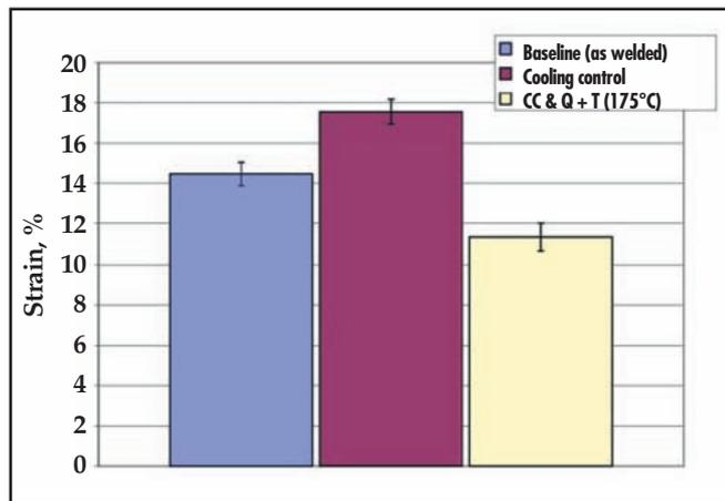
Fig. 16 — Comparison of maximum strains at fracture for seam-welded 28.6 mm diameter x 0.5 mm Type 410 SS tubing, average results for 16 trials.
