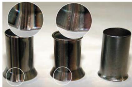
Fig. 18 — Typical ASTM A513 ring flare-test tube specimens; from left: as welded; cooling-controlled; CC Q+T hardened.
