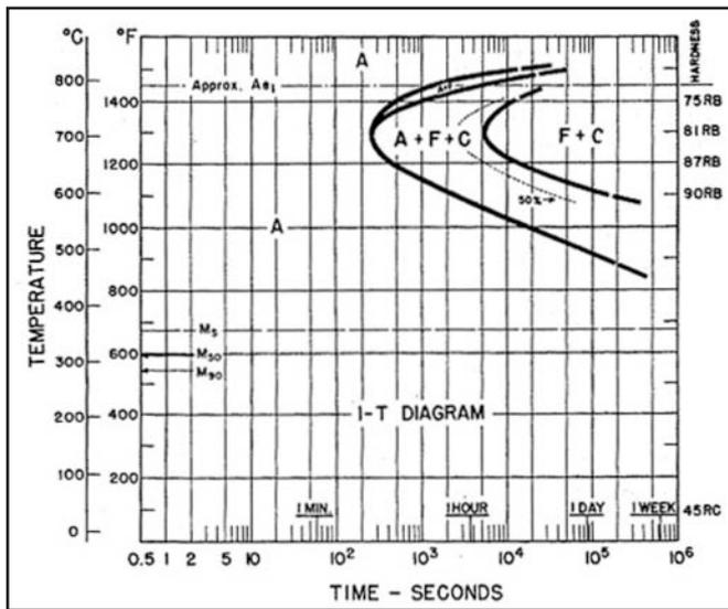
Fig. 9 — Time-temperature transformation (TTT) diagram for Type 410 stainless steel<sup>[6]</sup>.
