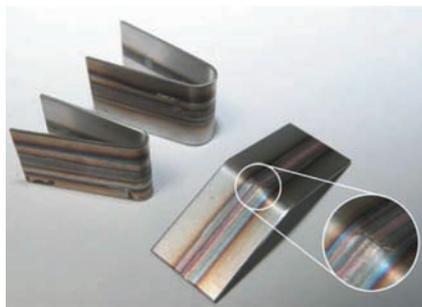
Fig. 4 — Typical ASTM E190 guided bend-test weld ductility specimens. From left:  $2t$  bend radius-full bend;  $4t$  bend radius-full bend;  $4t$  bend radius-failure.
