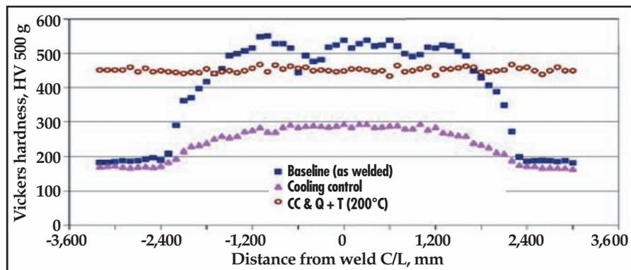
**Fig. 14 — Typical Vickers microindentation hardness profile; load: 500 g; hardness spacing: 100µm; seam-welded 19.1 mm diameter × 1.2 mm Type 410 SS tubing.**
